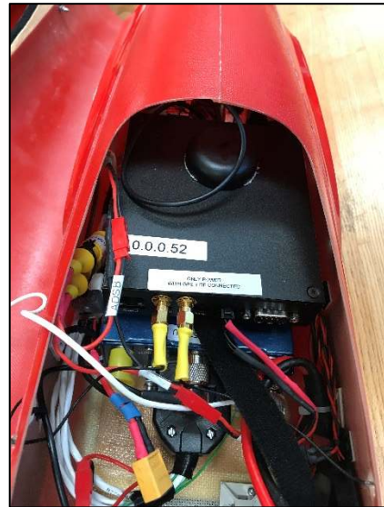
Figure 6 - Installation of the Unex OBU-201 in the Tempest.
