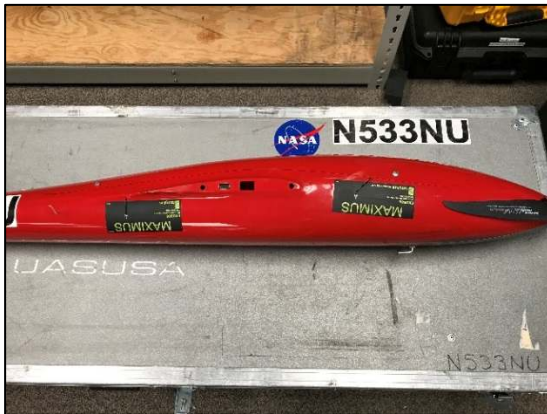
Figure 3 - Tempest fuselage illustrating installation of antennas for the Botlink (aft) and Unex OBU-201 (forward).
