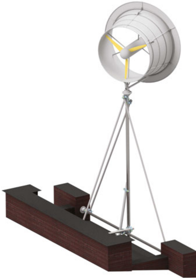
Figure 6. Roof-mounted SWT equipped with the diffuser.
