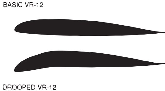
Figure 6. Sketch of the VR-12 profile used for wind tunnel testing at NASA Research Center from Lee paper [32].
