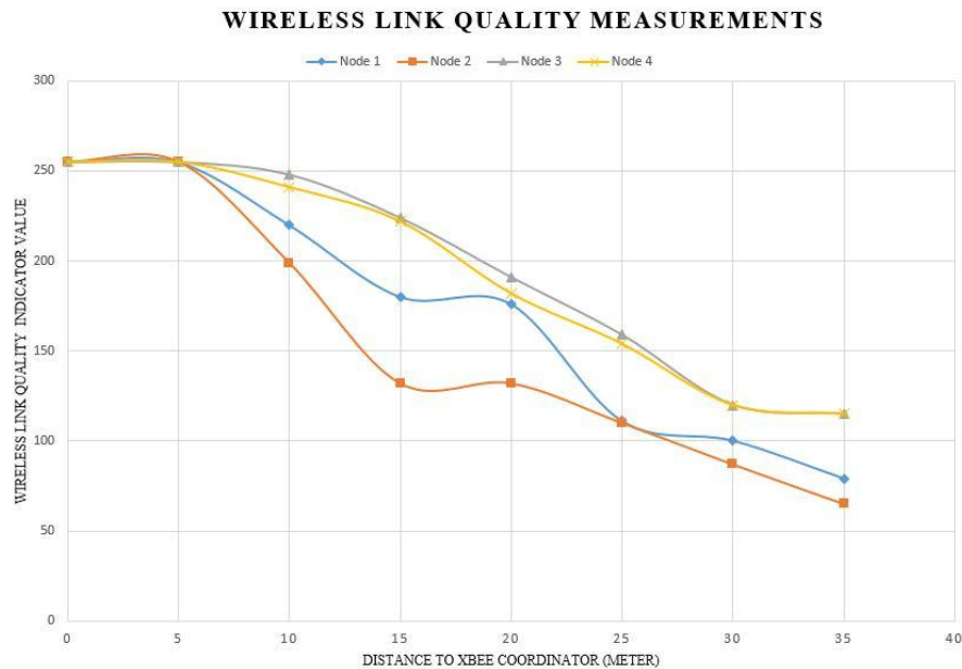
Figure 10. Wireless link quality measurements.
