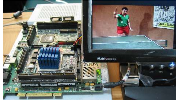
Fig. 6. Verification results of the H.264 decoder based on the proposed architecture using an FPGA prototyping board.
