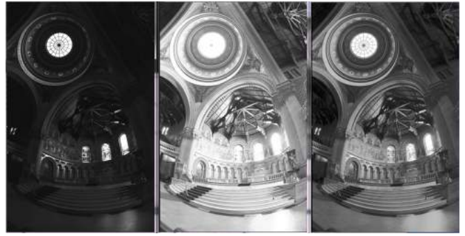
Fig. 6. Simulation of the global Duan et al. algorithm [36] in C++. Two consecutive exposures captured at immediate time steps t_1 , t_2 contain different luminance ranges of a scene. The result on the right is the tonemapped image.
