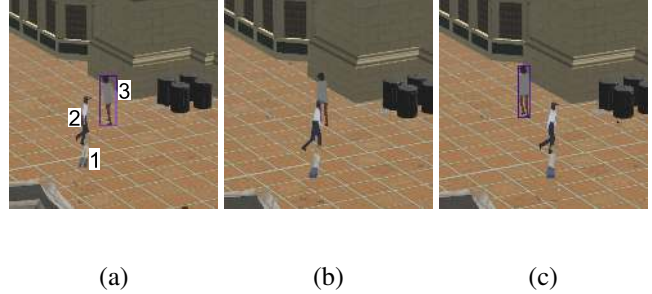
Figure 4: The LVRs are programmed to track pedestrians 1 and 3. Pedestrian 3 is tracked successfully; however, (a) track is lost of pedestrian 1 who blends in with the background. (b) The tracking routine loses pedestrian 3 when she is occluded by pedestrian 2, but it regains track of pedestrian 3 when pedestrian 2 moves out of the way (c).
