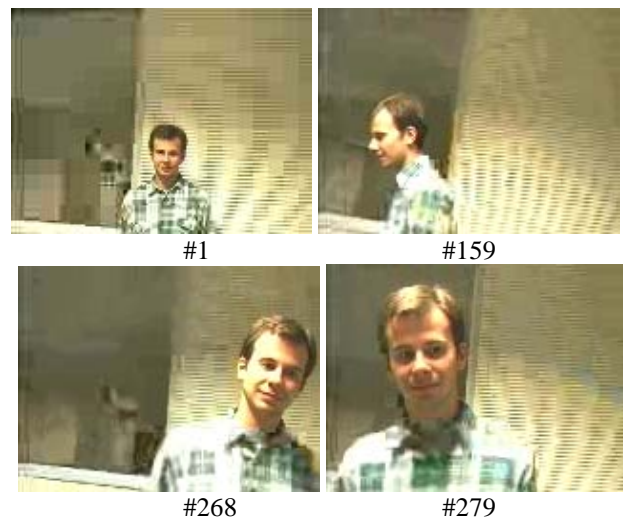
Figure 5. Reconstructed Alessio_2 sequence. Compression ratio is 53.74. The PSNR is 35.5 dB for the face and about 26dB for the background.
