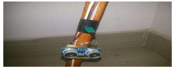
Figure-3: Smart Cane with Ultrasonic Sensor
