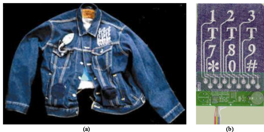
Figure 18. (a) Musical jacket. (b) Fabric keypad with circuit board placed behind it [89].
