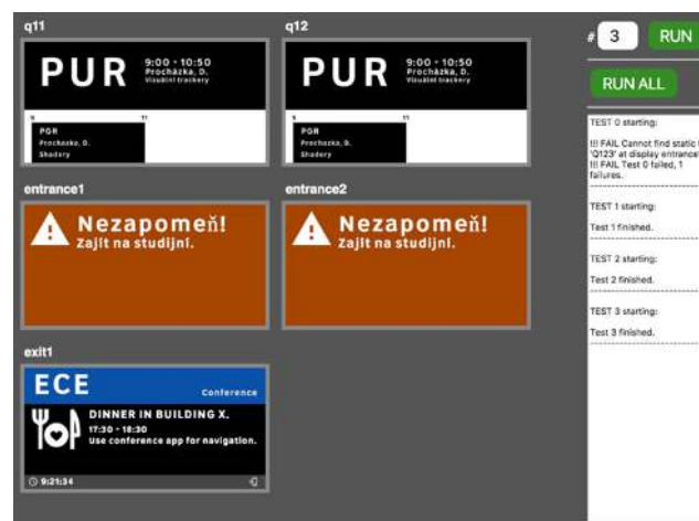
5: Fig. 5 Web-based tester of displays. For each predefined test, it passes test data and test environment including fake users to the server. Then it waits till all the displays are refreshed. Finally, it checks whether emulated displays contain the expected texts.
