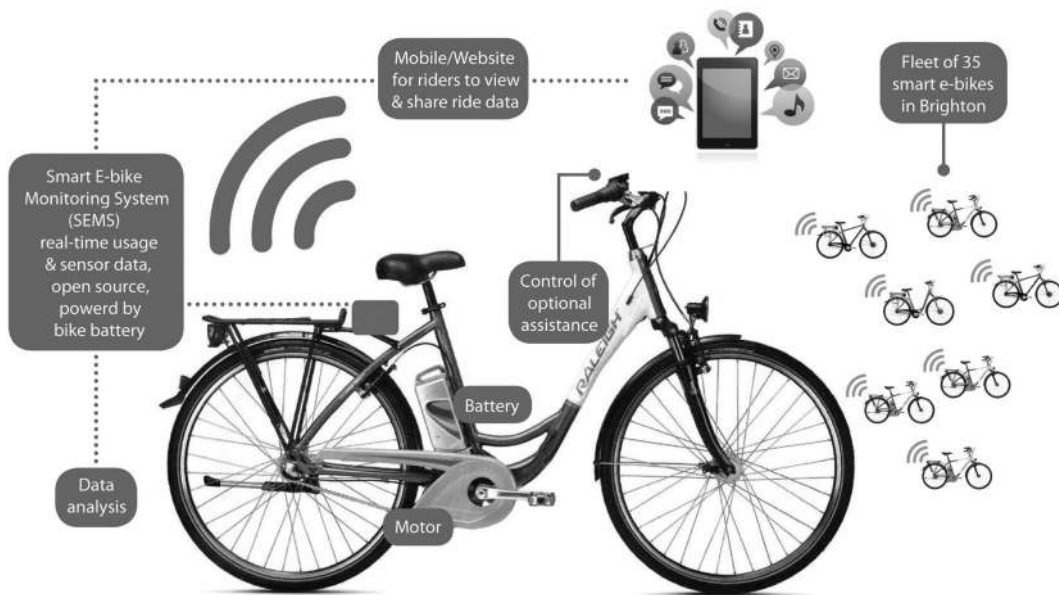
Fig. 2 SEMS was developed to collect real-time usage and sensor data, combining open source software and open hardware
