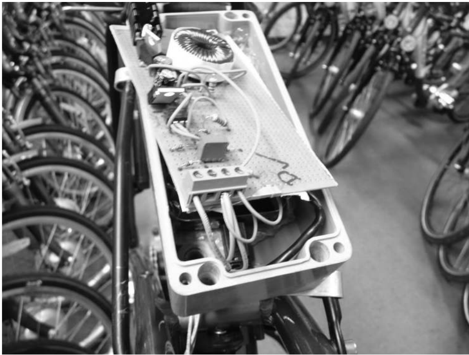
Fig. 6 SEMS electronics, the IOIO board and the Android phone are housed in a water-proof box and are wired into the e-bike battery
