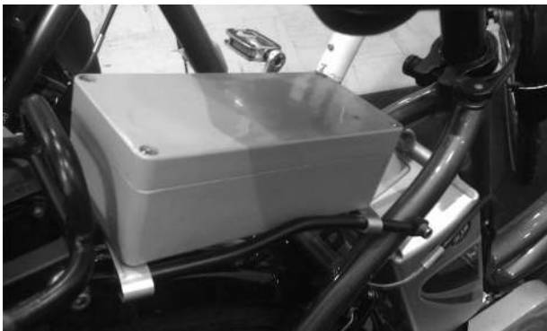
Fig. 5 SEMS electronics are housed in a water-proof box that is mounted under the saddle and fixed to the bike rack. No user interaction such as charging or switching on is required
