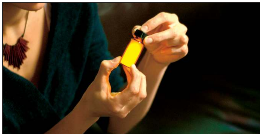
Figure 2. Shake-light bottle. Shaking the bottle collects energy, which is activated as light energy by removing the cap.
