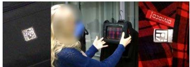
Figure 5: The fake tag reader on the handbag and fake RFID tag attached to a scarf. Here, the bag display matches the pattern of the scarf.
