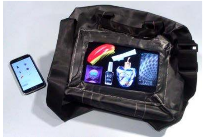
Figure 4: The remote control device (left) and an interactive handbag showing content inside it (right).
