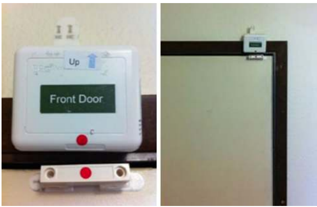
Fig. 7 An illustration of correct placement of the front door sensor: on the left , the two red dots should be aligned, and on the right is the proper way to place the front door sensor
