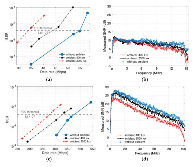
**Figure 9.** BER performance under ambient light for (**a**) headlamp at 100 lux and (**b**) measured SNR, and (**c**) BER performance under ambient light for blue LD beam at  $0.08 \text{ W/m}^2$  and (**d**) measured SNR.
