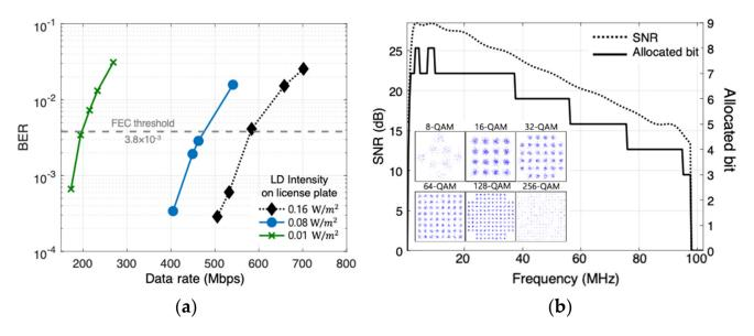
**Figure 8.** (a) BER performance according to output power of LD; and (b) constellations, measured SNR and allocated bits with adaptive bit and power loading.
