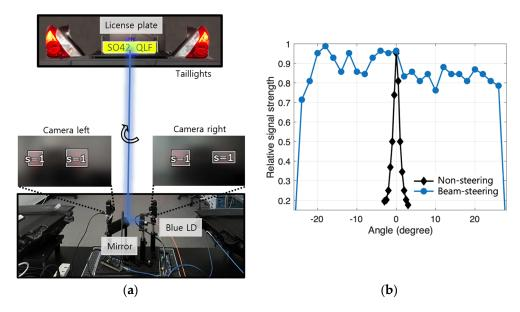
**Figure 6.** (a) Comparison of received signal strength with and without beam steering; (b) Beamsteering and tracking setup.
