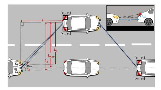
Figure 4. Geometric configuration for top and side views.
