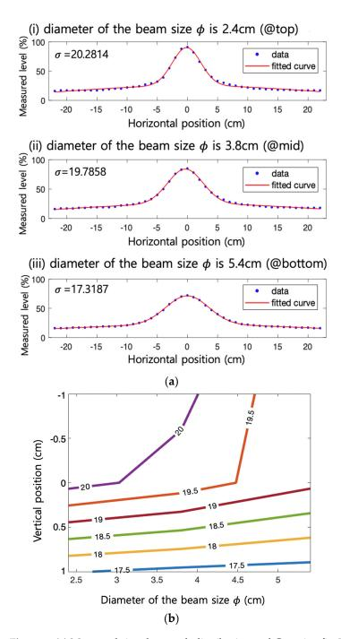
**Figure 5.** (a) Measured signal strength distribution and Gaussian fit; (b) overall standard deviation analysis.
