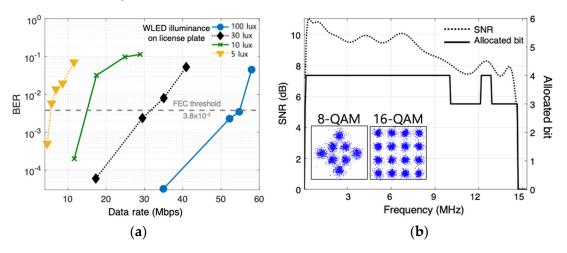
**Figure 7.** (**a**) BER performance according to different lux levels of LED headlamp; and (**b**) constellations, measured SNR and allocated bits with adaptive bit and power loading.
