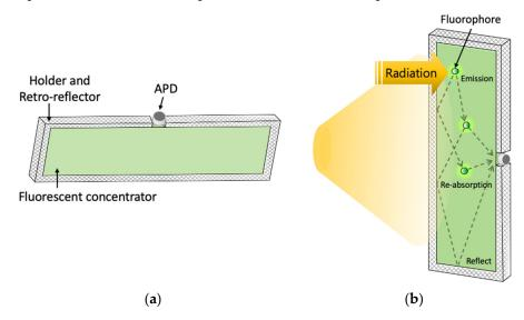
**Figure 2.** (a) Design of license-plate-shaped receiver; (b) schematic diagram of the physical process of a fluorescent concentrator.
