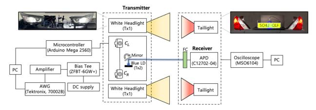
Figure 3. Schematic block diagram and experimental setup of the proposed V2V-VLC system.
