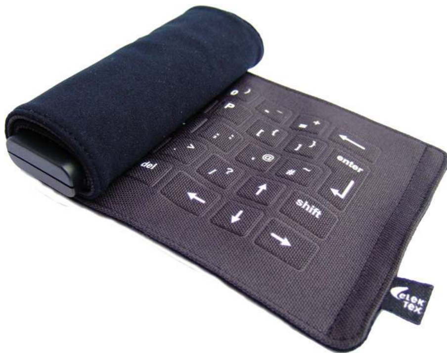
Figure 4. Elektext fabric-based keyboard (30 × 11 cm; weight, 65 g). (Courtesy of Eleksen.)
