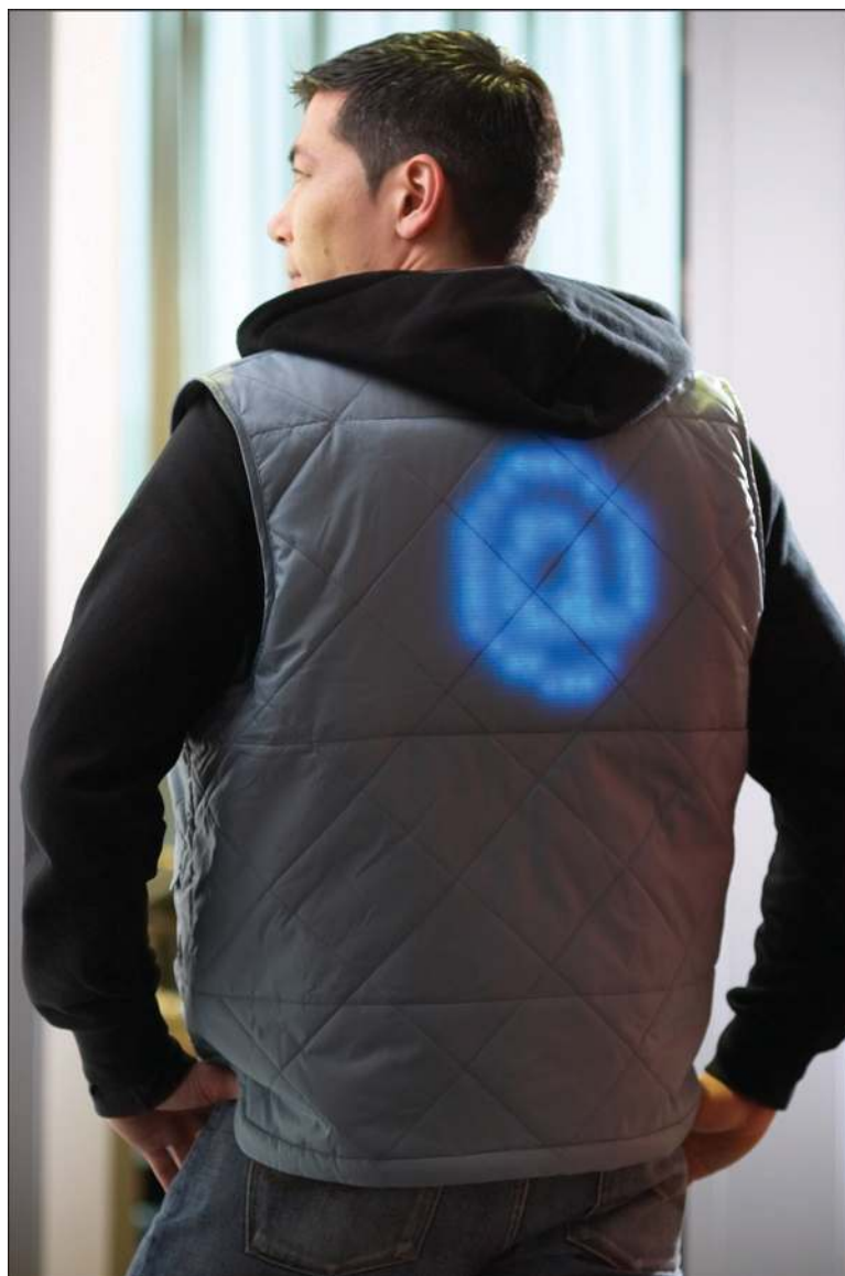
Figure 5. Lumalive textile garment from Philips features flexible arrays of colored light-emitting diodes fully integrated into the fabric. (Courtesy of Philips.)
