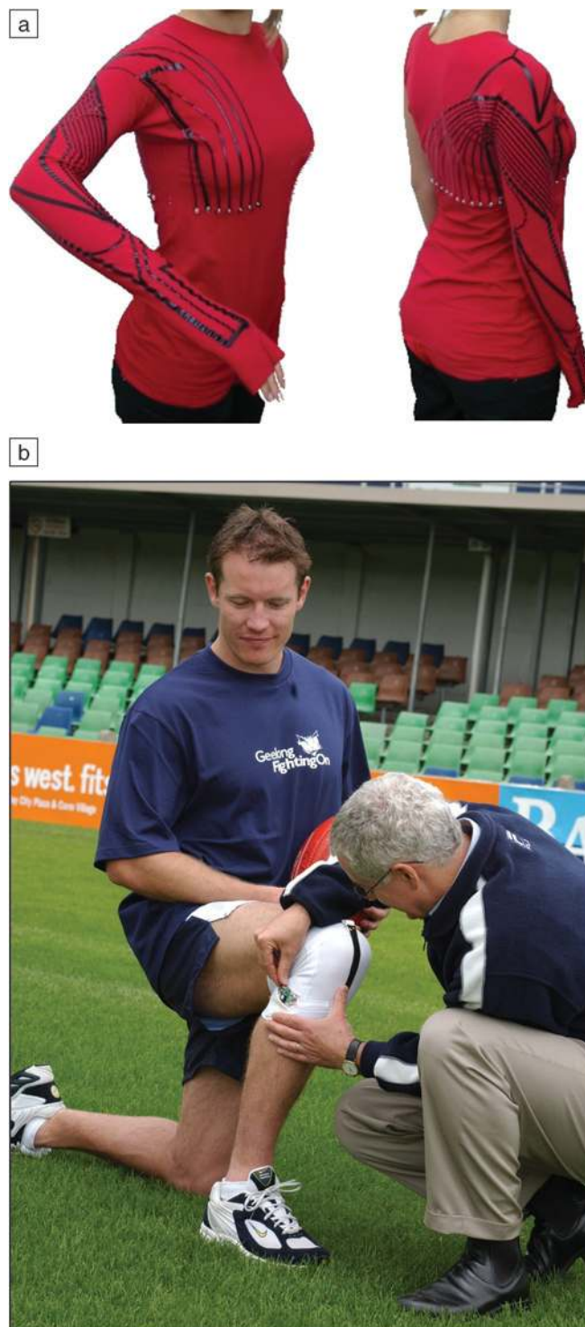
Figure 3. (a) Carbon-loaded elastomer-sensorized garment for kinesthetic monitoring developed at the University of Pisa. (b) The Intelligent Knee Sleeve is a biofeedback device using PPy sensors that monitors the wearer's knee joint motion. (Courtesy of CSIRO Textile and Fiber Technology.)
