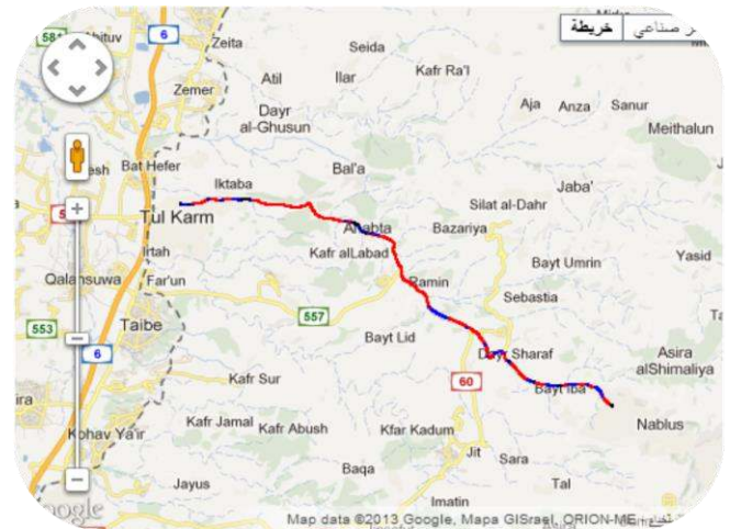
Figure 10. Nablus-Tulkarem Trip. The picture above is automatically generated by the system. The Map source is Google Maps [5]. The red line represents the trip path. This path is generated through the insertion of GPS module readings into Google Maps. The blue lines depict the locations where the vehicle driver exceeds the threshold speed.
