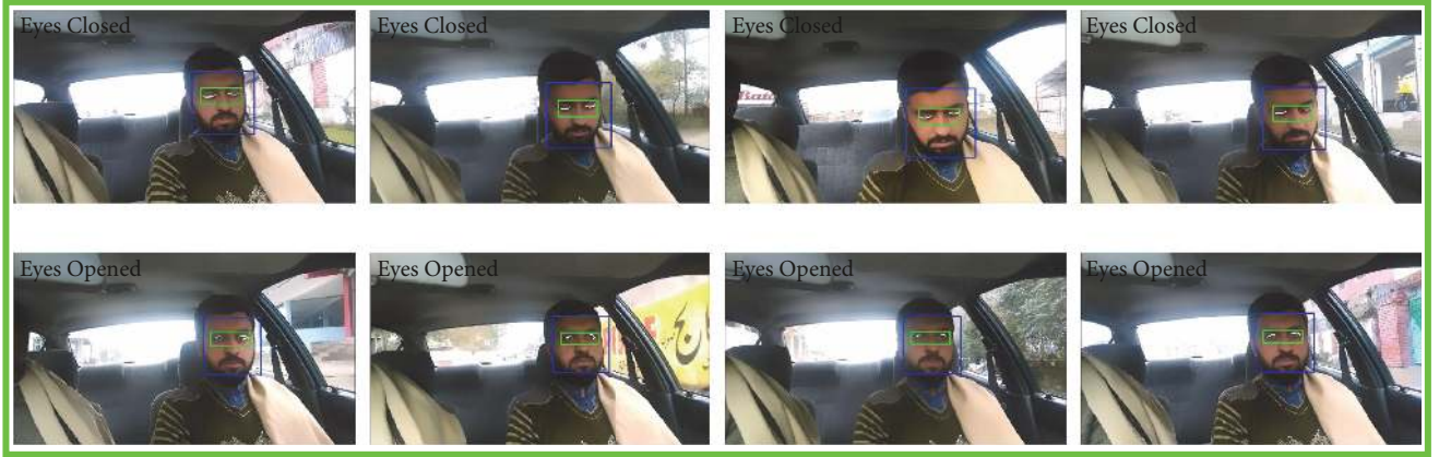
FIGURE 13: Correct detection of open and closed eyes on the video dataset.
