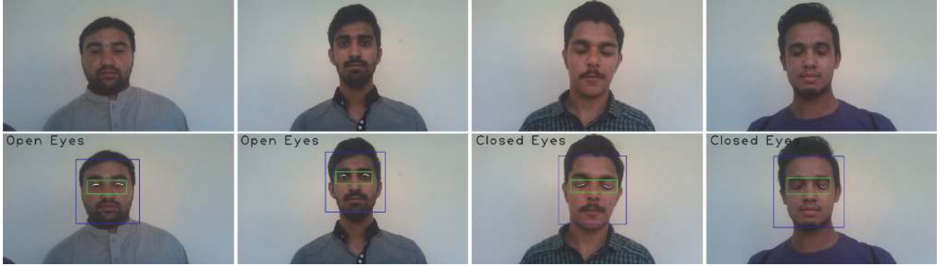
FIGURE 10: Detection results of open and closed eyes from images with a homogeneous background.
