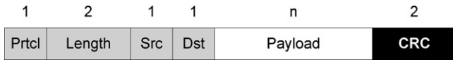
Fig. 3. NanoUDP message format. Prctl is the protocol and flag byte. Length is the total length of payload and possible CRC. Src and Dst are source and destination port numbers, both 0×28 for SSI. CRC checksum is used if requested by the application.
