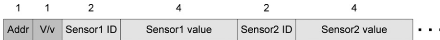
Fig. 5. SSI sensor data response ‘V’ message. All the sensor values requested are sent. Addr is the device address, one byte, followed by the message type ‘V’ or ‘v’. After that, the sensors’ values requested with ‘R’ or ‘r’ command follow.
