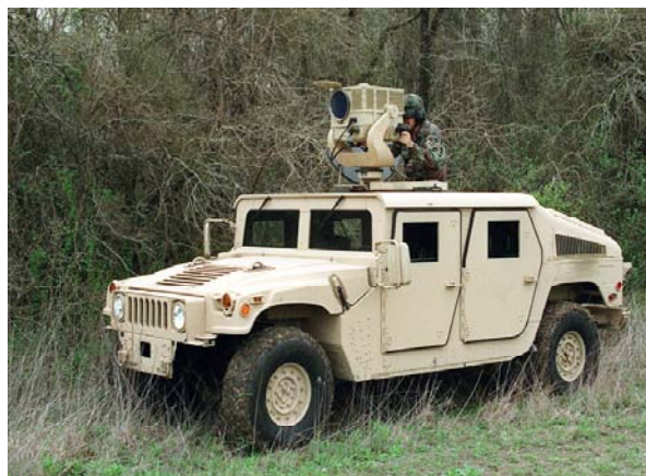
Figure 6 : Long Range Advanced Scout Sensor System will incorporate ATR to aid in Search and Track
