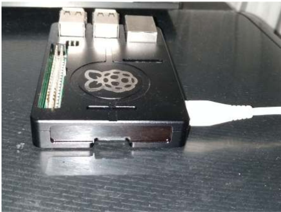
Fig. 5 Raspberry Pi (Edge Gateway)
