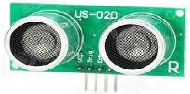
Figure 11. Physical representation of ultrasonic sensor
