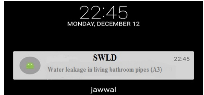
Figure 30. Result when leakage detected in region 4
