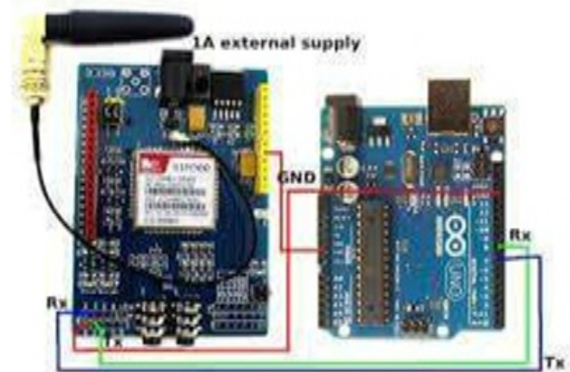
Figure 8. Connect the GSM 900 with Arduino mega
