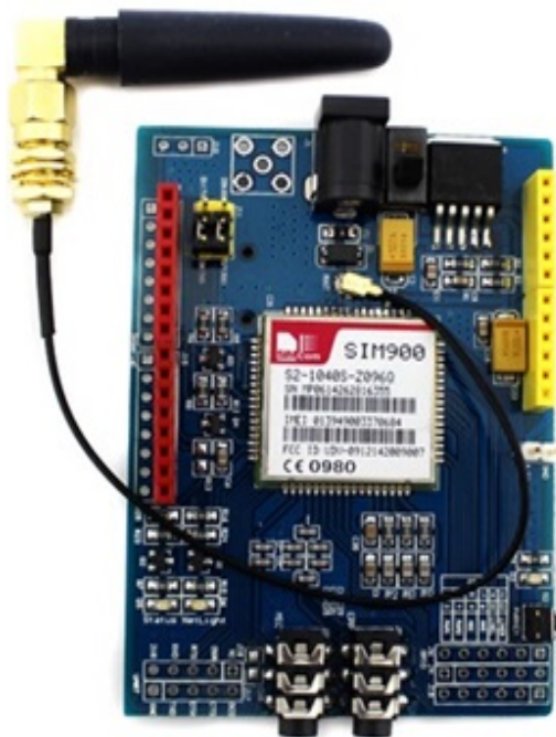
Figure 7. SIM900 for Arduino controller
