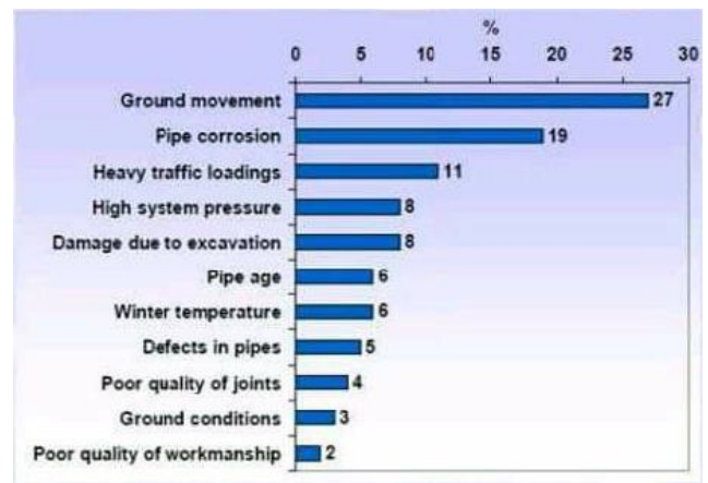
Figure 35. Percentages to the factors that causes leakage
