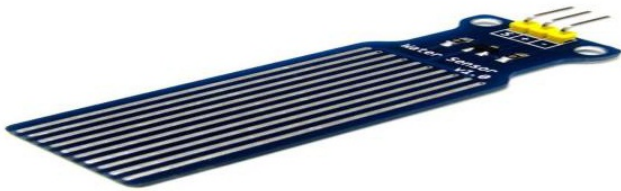
Figure 9. Physical representation of water sensor
