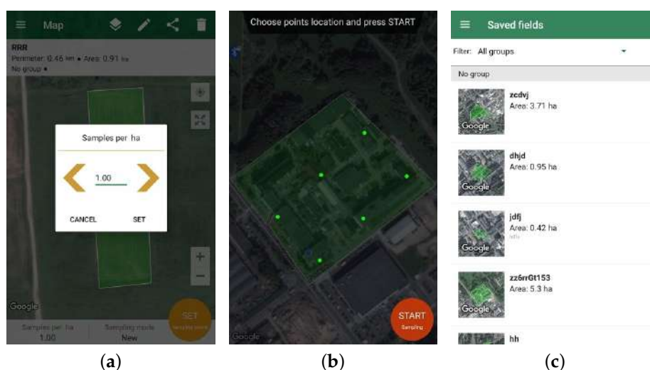
Figure 33. Soil Sampler: (a) Setting the desired number of samples; (b) Sample location visualization; (c) History of saved fields.
