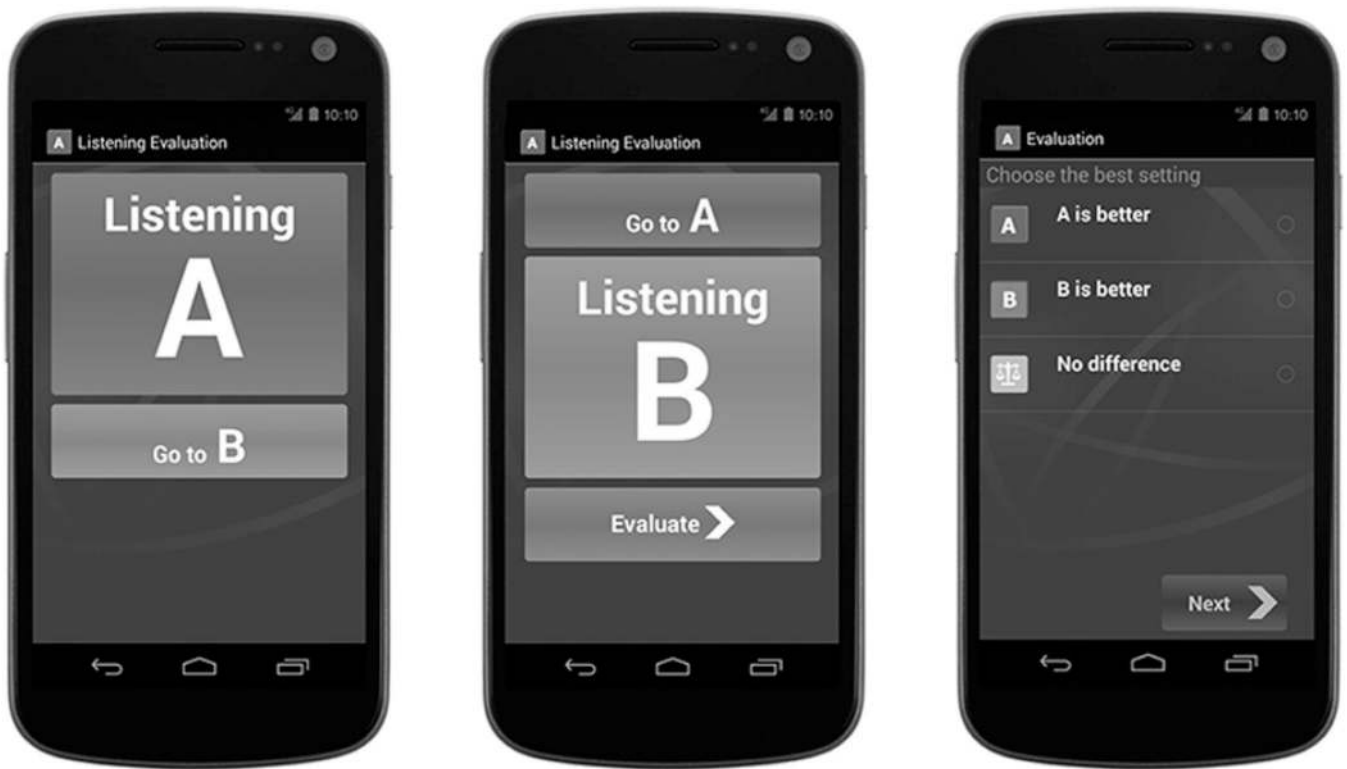
Figure 2. Smartphone screen shots of the A/B Test sequence: Listening to setting A (left), listening to setting B (center), and choosing the best setting (right).
