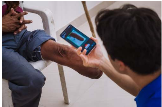
Fig. 1. Image of an amputee's limb being scanned with a beta version of the authors' implemented cellphone application.
