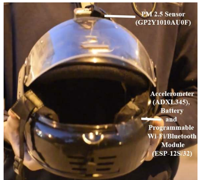
Figure 7. The helmet in its final prototype state. A part of this image is deliberately blurred to avoid intellectual property rights violation.
