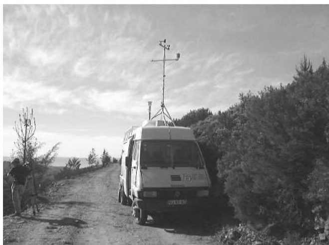
Fig. 2. Photo of van 2 and its air quality equipment.
