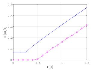
**Figure 17.** Real linear velocity, while the robot Pioneer 3DX is following the trajectory (magenta line), deviates from the applied linear velocity (blue line).
