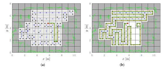
**Figure 9.** The RSTC algorithm in the *Lab scenario* with the presented RSTC spanning tree (blue line), the RSTC path (black line), the smoothed path by the SCCPP algorithm (red line), and the executed path by the smoothed RSTC algorithm (green line). Red points are the robots' position where the replanning algorithm is executed. (**a**) The smoothed RSTC path in the *Lab scenario* before replanning. (**b**) The smoothed RSTC path in the *Lab scenario* after replanning.
