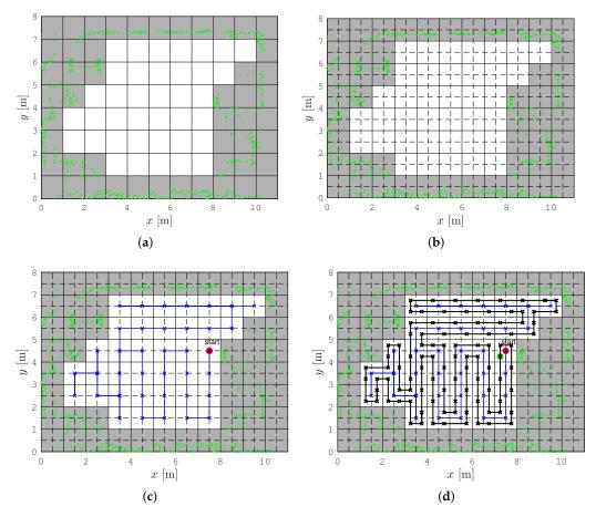
**Figure 3.** Example of the complete coverage path planning for the known environment step-by-step. The real obstacles collected by SLAM algorithm are presented with green dots. (**a**) Low resolution occupancy grid map, (**b**) Subdividing of grid cells, (**c**) The spanning tree (blue line), (**d**) Complete coverage path (black line).
