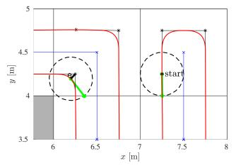
**Figure 5.** The enlarged part of the coverage path with two positions of the robot: (1) the robot's starting position and (2) the robot's position at the obstacle corner. The obstacle cell is shown in gray, the robot's positions in dashed circles, the robot's orientation in green, the spanning tree in blue, the RSTC path in black, and the smoothed path in red.
