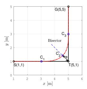
Figure 4. Illustration of the sharp turn smoothing by two clothoids.
