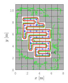
**Figure 15.** The calculated SCCPP path (red line) and trajectory tracked by the Pioneer 3DX robot (green line).
