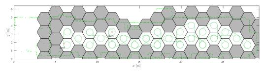
Figure 13. The complete coverage of the HDCP algorithm with hexagonal cell grid.
