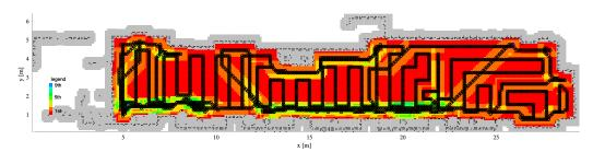
**Figure 12.** The complete coverage of the CCD\* algorithm with the path and noted redundant numbers of cell visits (from 1 to 9).
