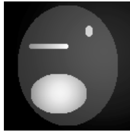
Figure 2. The result of the phantom in figure 1 filtered by a 3x3 median filter.
