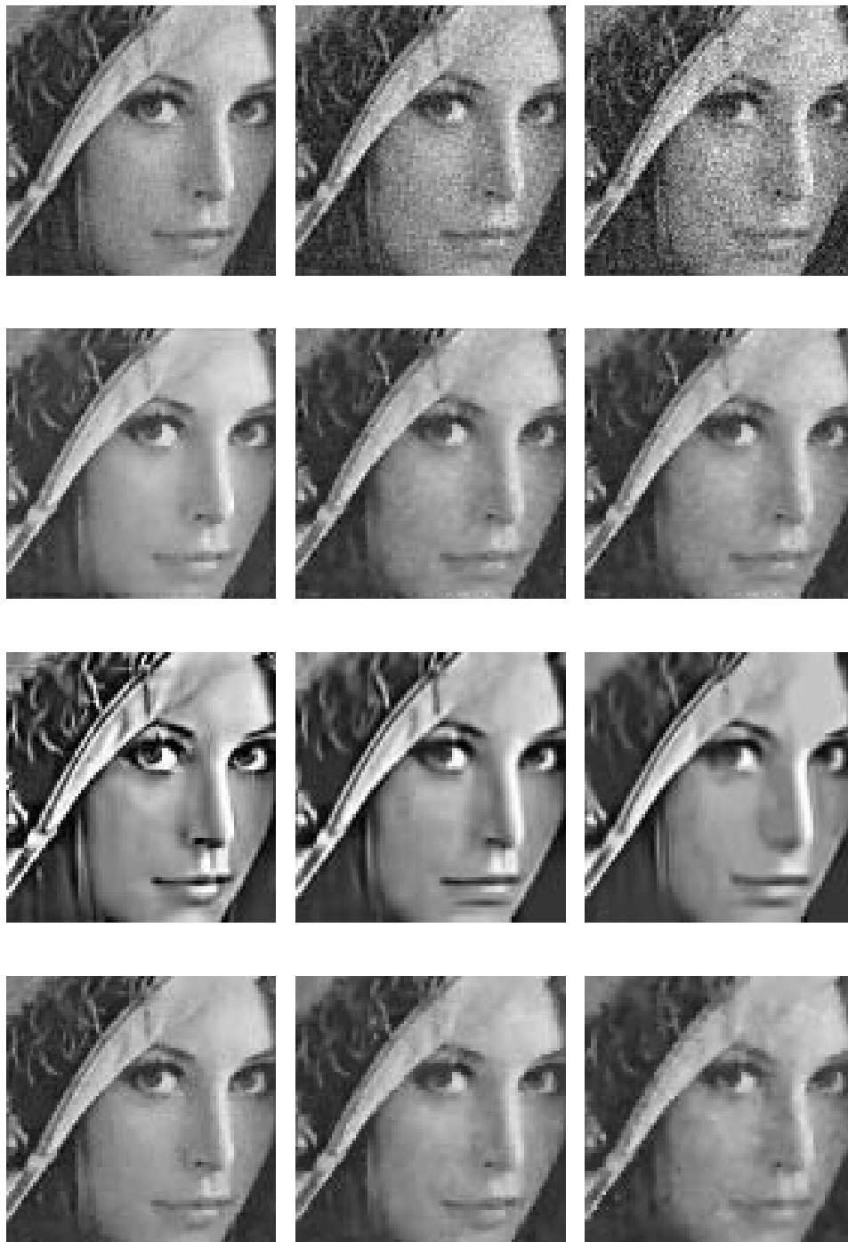
Fig. 12 First row, Lenna image corrupted by Gaussian noise with standard deviations \sigma = 10 , \sigma = 20 and \sigma = 30 . Second row, the output of Fuzzy Network filter. Third row, output of BM3DShar and in the last one, the output of TeD-FAB.
