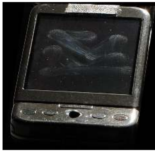
Figure 5: Phone A, from Experiment 1, where the pattern is entered with normal touches. Notice that the directionality of the pattern can be determined at ever direction change.
