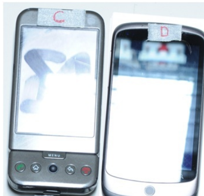
Figure A4: An image from Experiment 1: Complimentary lighting and lens angle causes significant glare, leading to unidentifiable patterns and information loss.
