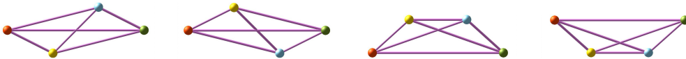
Fig. 2. Local minima: The two undeformed realizations G(\mathbf{V}_1) and G(\mathbf{V}_2) and the two deformed stable realizations G(\mathbf{V}_3) and G(\mathbf{V}_4) (from left to right). The point A is colored red, B green, C blue and D yellow, respectively. This color-coding is also used in the Figs. 3–5.
