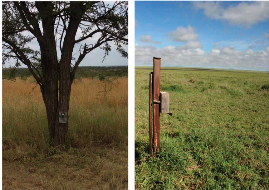
Figure 2. Camera trap placement. Camera traps in steel cases were placed on trees when available (left, n = 195 ) and steel poles when no trees were within 1,000 m of the grid-cell centre (right, n = 35 ).
