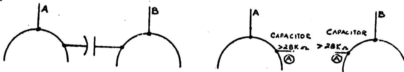
FIGURE 3-6. High Impedance Sub-Tree Partitions
