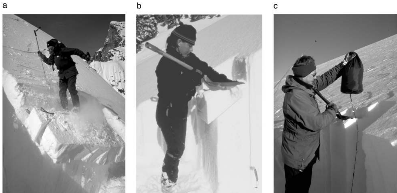
Figure 14. In situ snow slope stability testing usually involves isolating a snow block including a weak layer and loading the block at given steps: (a) rutschblock test, (b) compression test, and (c) stuff block test [from Schweizer and Jamieson, 2003a].
