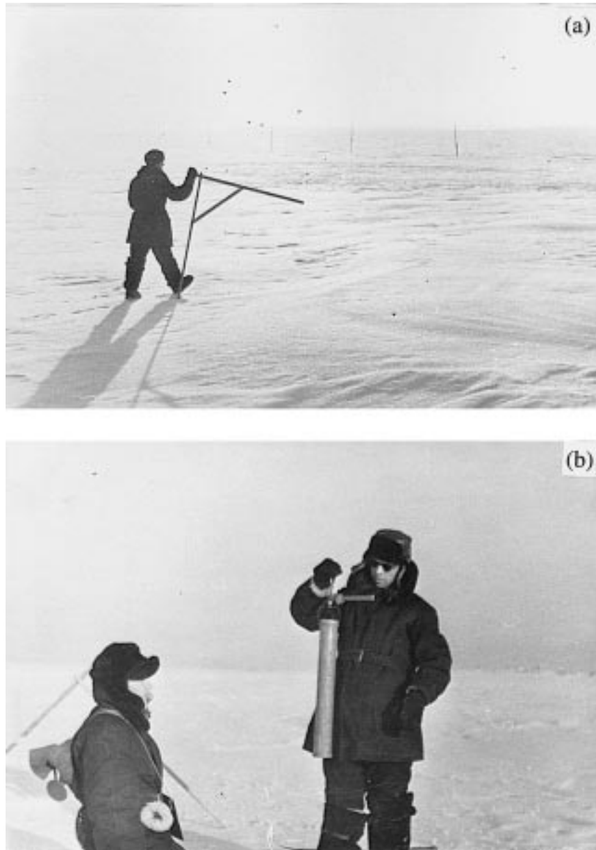
FIG. 2. Photographs at station NP-6. (a) Measuring distance along a snow line. (b) Weighing snow to obtain its density. (Photographs by N. N. Bryazgin, 1957.)
