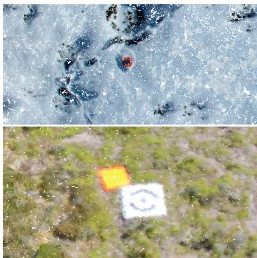
Figure 6. Bootstrap validation was done by finding the photo identifiable control points in the reconstructed point cloud (shown above), and comparing the estimated coordinates with those measured from RTK GPS.
