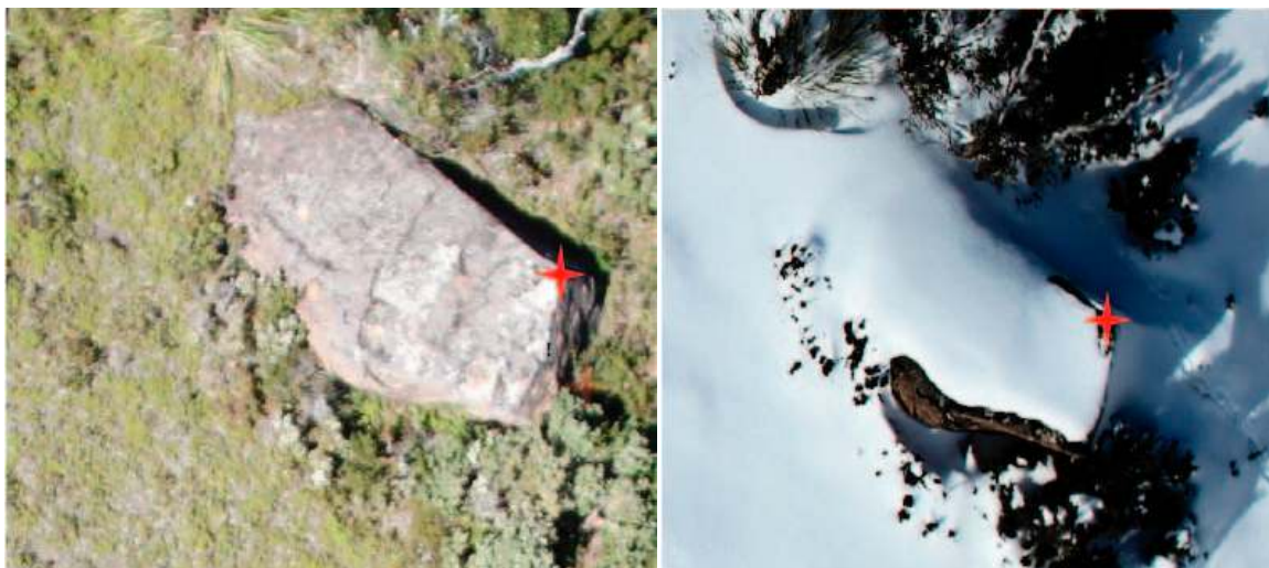
Figure 9. For co-registering the two datasets, we used the corner of a large boulder (red star) within the study site to estimate the translational components for the affine transformation.
