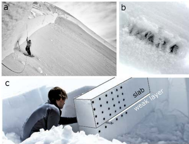
Figure 1. (a) Crown fracture of a dry-snow slab avalanche in Mt. Baker, USA (©Grant Gunderson). (b) Surface hoar weak layer. (c) Propagation saw test. The weak layer is represented in white, the slab in grey. The black dots are markers used for particle tracking to measure slab deformation.
