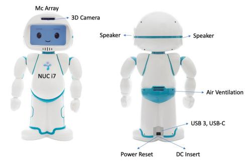
microphones to recognize where the sound is coming from and speakers which allow the robot to produce verbal communication or play sounds.
