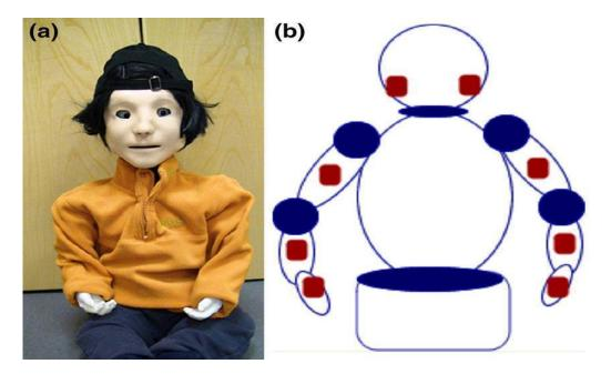
Figure 5. KASPAR robot (a) and sensors localization (b).
