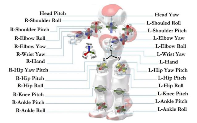
Figure 1. Localization of stepper-motors inside NAO robot.
