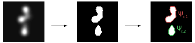
Fig. 5. Computation steps for contour extraction and grouping, namely (from left to right), sociality density, thresholding and contour detection.
