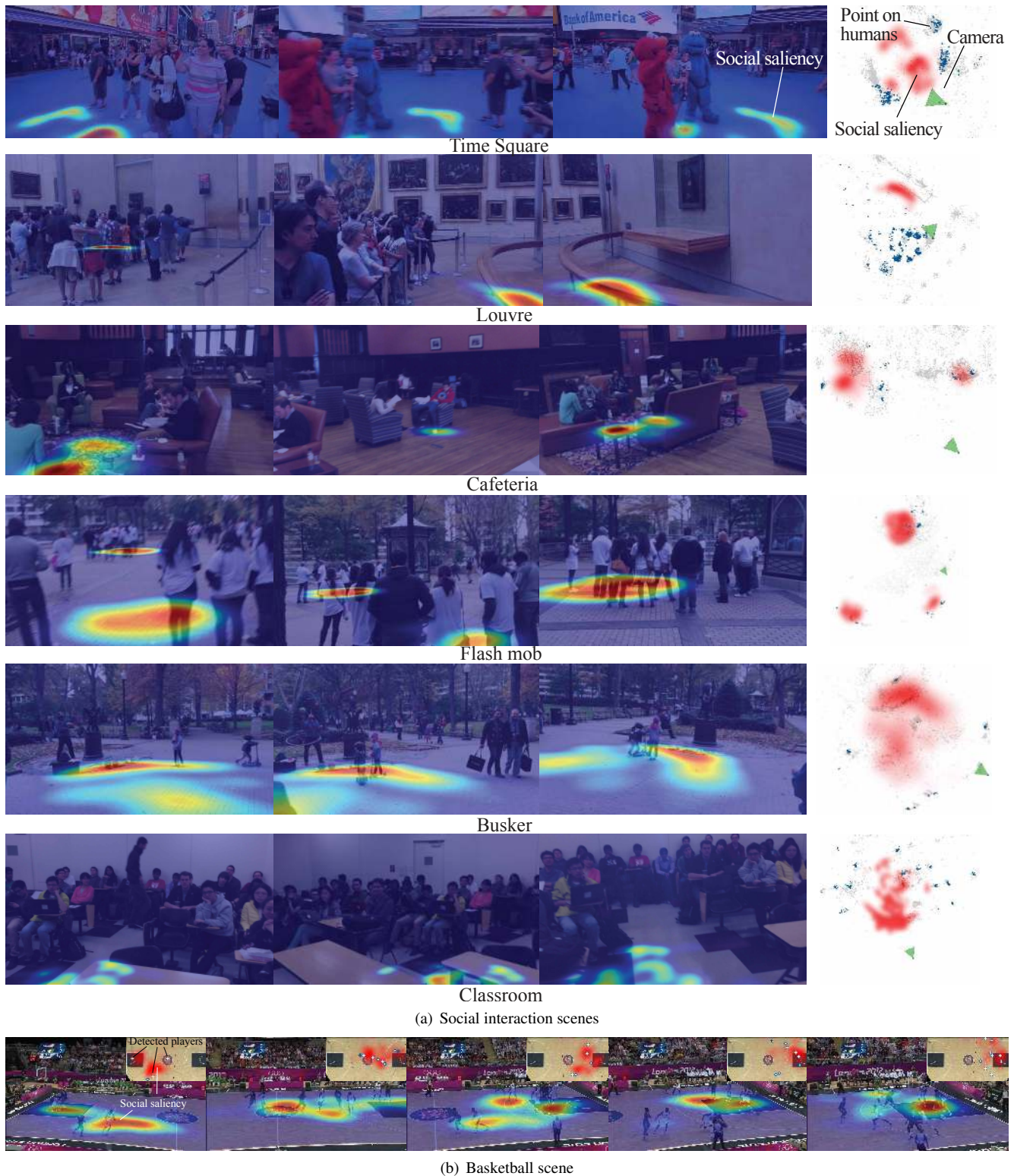
Figure 5. We apply our method to predict social saliency on third person videos. (a) We identify social space (space around the photographers and subject with the Muppet characters and space near Mona Lisa painting) in the Time Square and Louvre scenes obtained from YouTube. Multiple social groups are detected in the Cafeteria and Flash mob scenes. In the Busker and Classroom scenes, joint attention forms around the busker and podium. (b) We use the modified social formation feature to predict social saliency in a basketball game.
