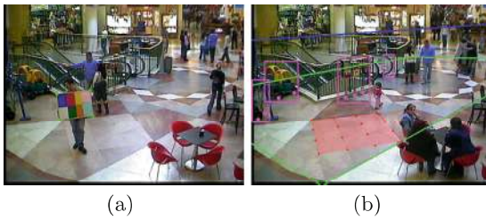
Fig. 1. (a) Detected chessboard points for camera calibration; (b) Horizontal vanishing line (blue), ground plane's projection area (green), ground points (red) to calculate scale factors and reprojection errors, and objects of interest (purple) (Color figure online).
