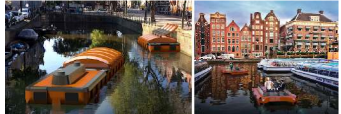
Fig. 1. Roboat: Robotic boats designed to serve as a platform for trash removal and as a new means of transportation in Amsterdam canal.
