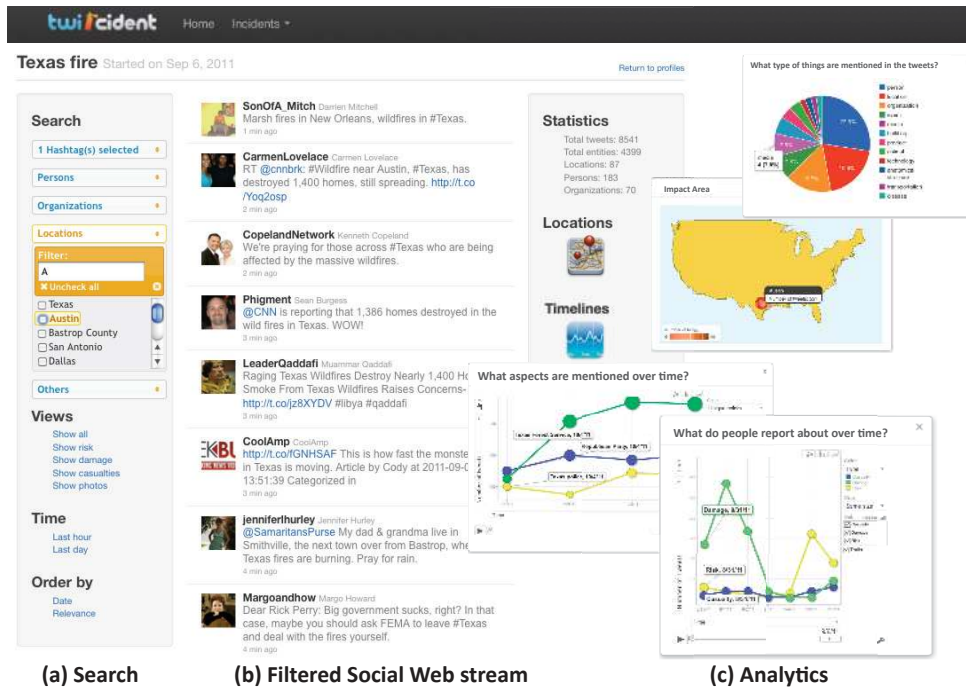
Figure 6.2: Screenshot of the Twitcident system: (a) search and filtering functionality to explore and retrieve particular Twitter messages, (b) messages that are related to the given incident (here: fires in Texas) and match the given query of the user and (c) real-time analytics of the matching messages.
