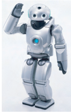
Fig. 1. QRIO, a small humanoid robot prototype was used as the research platform.
