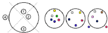
Figure 2. A schematic of the social proxy and, to its right, three instances of it. The schematic shows two people (dots 1 & 2) actively involved in a conversation, one inactive person (dot 3), and one person involved in a different conversation (dot 4). Each dot occupies a (virtual) wedge; wedges are created and destroyed as people log on and off. The first instance shows a 'hot' conversation; the second, a dormant one; the third a mixture of activity, idleness, with three people in other conversations.
