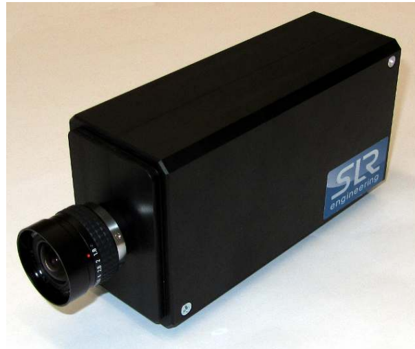
Fig. 5. The smart camera platform. A custom-built camera running Linux on a 1.6GHz Intel Atom processor with 2 GB memory and 100 MBit Ethernet interface. The image sensor is a CCD colour image sensor with a native resolution of 1280 \times 1024 pixels.
