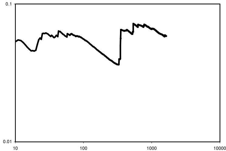
Figure 11: The cumulative variance of log changes in daily domestic water consumption (litres per day) in a metered UK neighbourhood (derived from the figures illustrated in figure 1 above).
