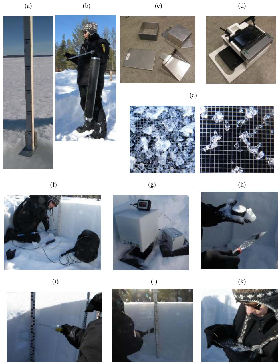
Figure 3. Photos of snow pit measurements: (a) tool for ice thickness measurements, (b) bulk SWE measurement with SWE tube, (c) box sampler and wedge sampler for density profile, (d) camera and stand for macro-photography, (e) two examples of snow grains on 1 mm grid, (f) SnowFork, (g) IceCube, (h) snow sample preparation for IceCube, (i) temperature measurement, (j) determining layers with brush and (k) definition of grain size and type in field.
